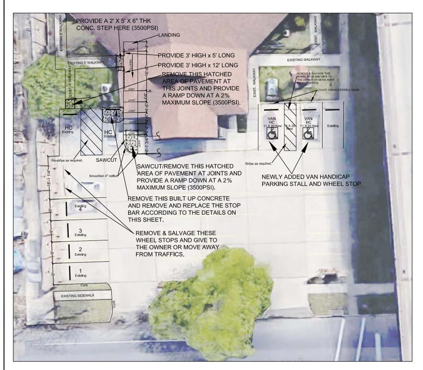
THE VAN ACCESSIBLE SIGN SHALL BE MOUNTED 60" MINIMUM ABOVE THE FINISH FLOOR OR GROUND SURFACE MEASURED TO THE SIGN BOTTOM AND ALL HANDICAP SYMBOLS MUST BE WHITE ON A BLUE BACKGROUND
